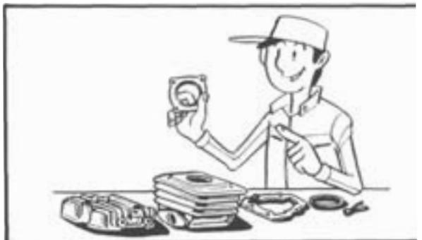
3. During engine disassembly, clean all parts and place them in trays in the order of disassembly. This will speed up assembly time and help assure that all parts are correctly reinstalled in the engine.
