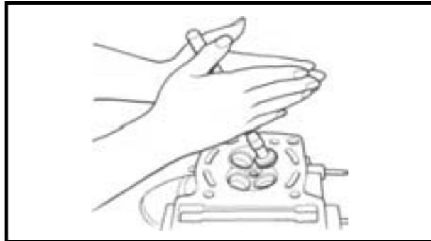
**Valve/Valve Seat Assembly Lapping**
