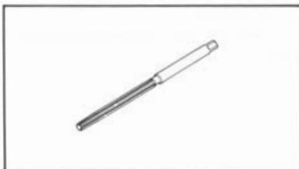
5. Valve Guide Reamer (5.5 mm)
